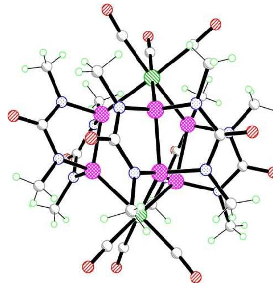
Solved, refined (to  $R1 = 3.8\%$ ) and published (JCS Dalton) in the space group  $I4_1/acd$  that is uniquely determined from the systematic absences. A crystallographic twofold axis lies perpendicular to the Mo...Mo vector, but the molecule also appears to possess a threefold axis along Mo...Mo.
